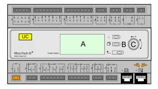
The keypad/display (A) consists of a 5-line by 22 character display.
