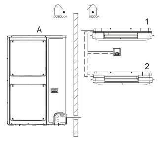
A Pair system or simultaneous operation system
