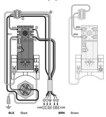
2 Make sure to ensure strain relief of the cable by correct use of the PG nipple and PG nut (mounted on the domestic hot water tank).
