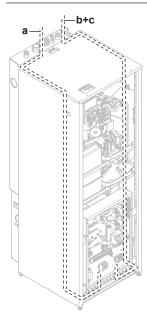
4 Fix the cable with cable ties to the cable tie mountings to ensure strain relief and to make sure that it does NOT come in contact with the piping and sharp edges.
