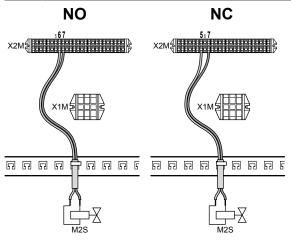
2 Fix the cable with cable ties to the cable tie mountings.
