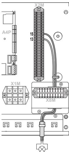
2 Fix the cable with cable ties to the cable tie mountings.
