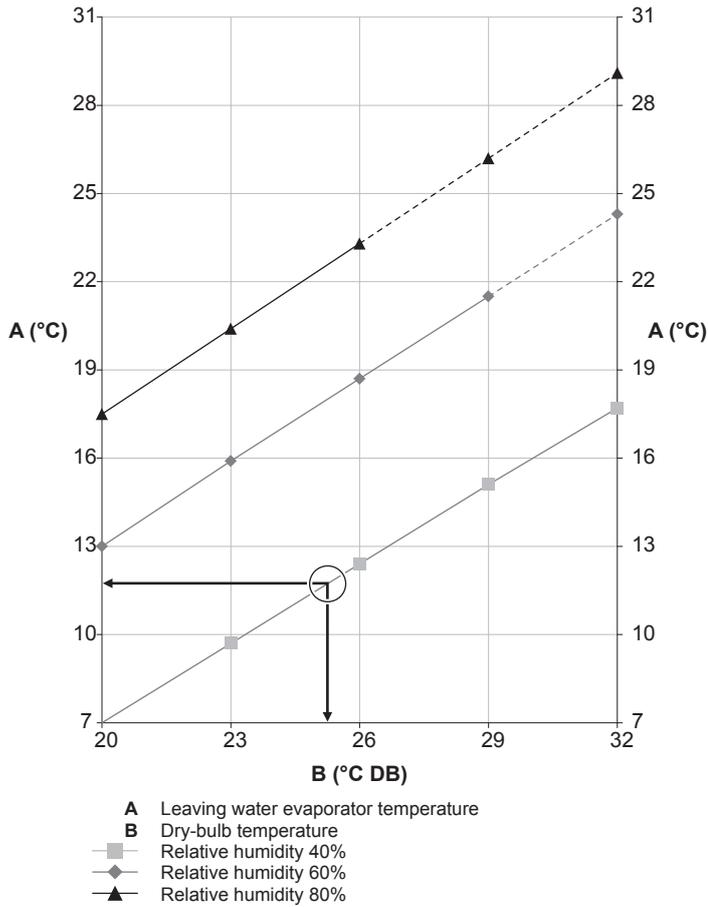
**Example:** Given are an ambient temperature of 25°C and a relative humidity of 40%. If the leaving water evaporator temperature is <12°C, condensation will occur.
