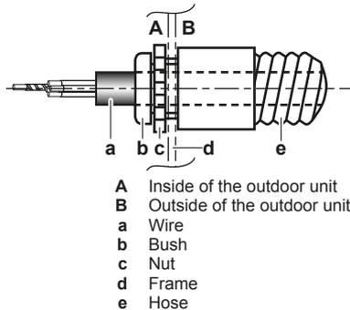
4 Inside the unit, route the wiring as follows:
