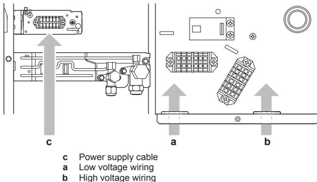
5 Make sure that the cable does NOT come in contact with sharp edges.
