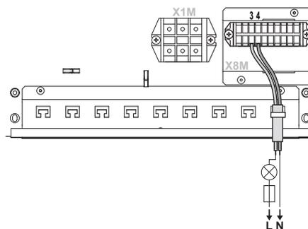
2 Fix the cable with cable ties to the cable tie mountings.
