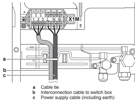
2 Open the switch box and route the wiring as follows.
