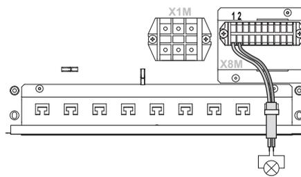
2 Fix the cable with cable ties to the cable tie mountings.
