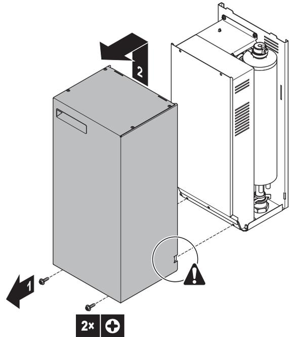
7.2.7 To open the switch box cover of the backup heater
