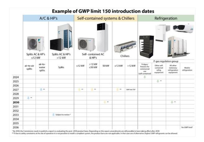
Example of cut-off dates for systems with a refrigerant with a GWP limit of 150 defined in the F-gas regulation EU 2024/573. © Daikin
